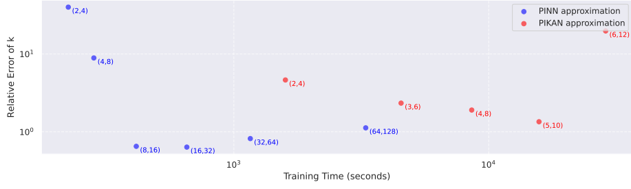
Fig. 13: log log plot of PINNs and PIKANs approximation on a semi-infinite domain. PIKANs tend to take much more to approximate a worse solution
